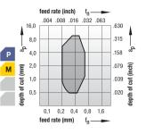
MR For medium to light roughing of steels, difficult-to-machine high-alloy titanium, and aluminum materials. High strength to deal with heavy chip deformation.
