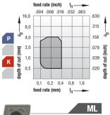
For finishing to medium machining with a negative, stable cutting edge.
