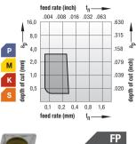
For finishing to medium turning operations with optimal chip control over a wide range of cutting conditions and workpiece materials.
