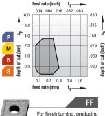
For finish turning, producing smooth, accurate surfaces. Very good chip control, especially at low depths of cut.
