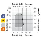
UM For medium-duty turning operations. Soft-cutting chipbreaker. Used in applications producing varying chip sections, such as profile or copy turning. Good dimensional accuracy. For soft steel materials and stainless steels.
