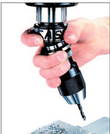
3. Removing drill chuck holder with one hand.
