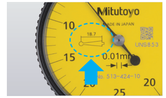
Contact point length is printed on dial face to avoid accuracy issues
